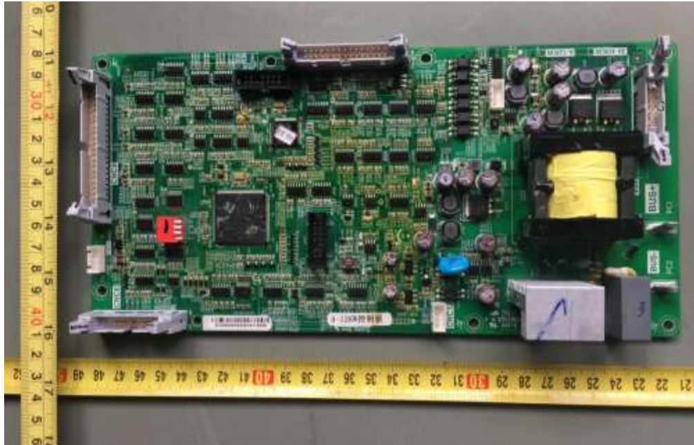
Front side of Control board
